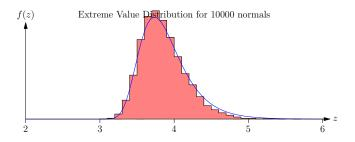
The Weibull distribution is used here to give a probability that a value is an maximal value from a normal distribution. With more samples, the distribution is more clearly defined.
